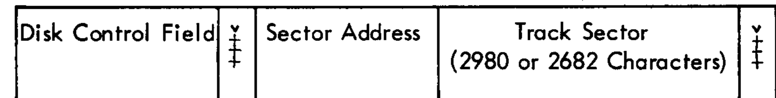
Figure 11. Core Storage Layout--Write or Read Track Record with Address
