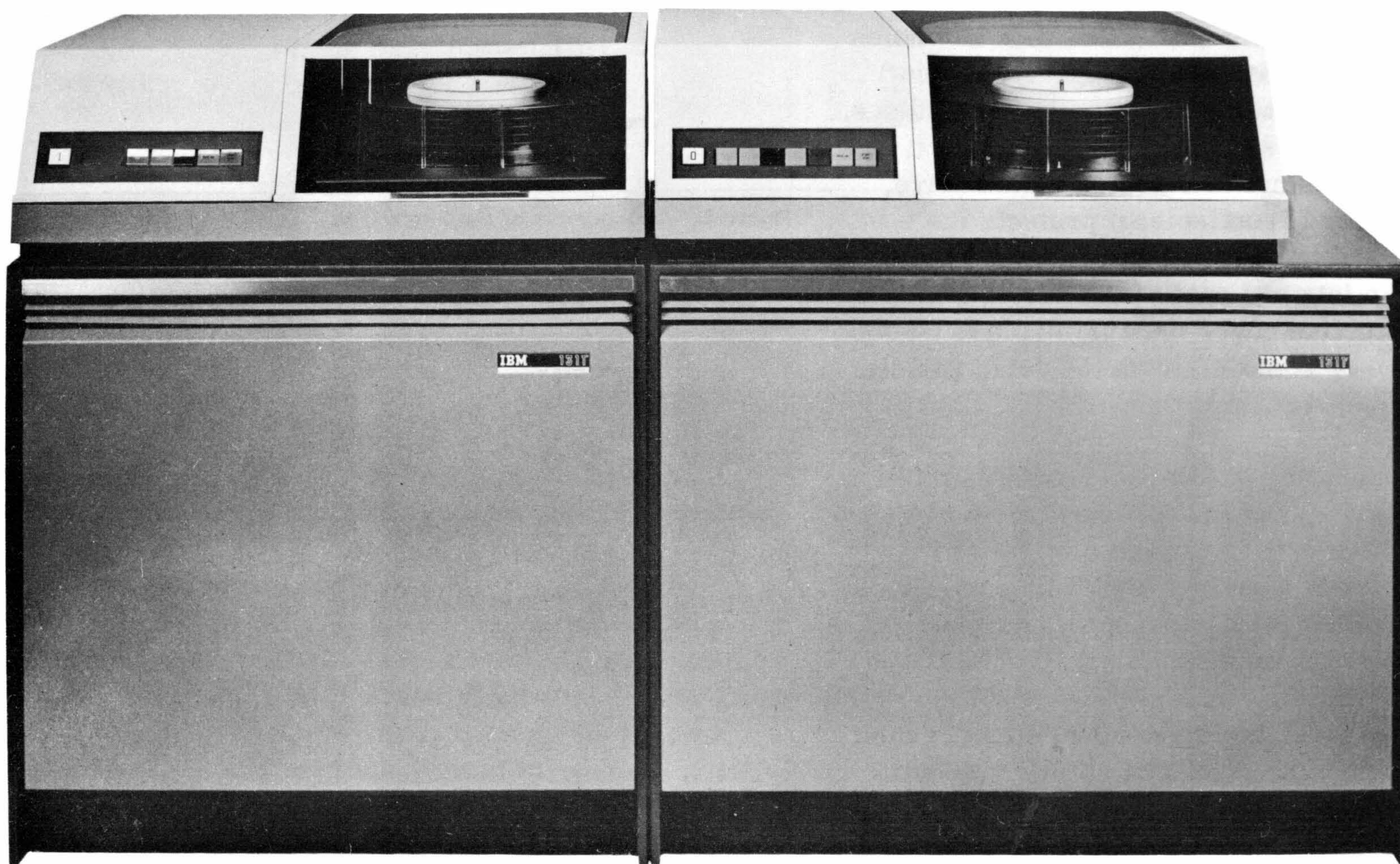
Figure 1. IBM 1311 Disk Storage Drives
